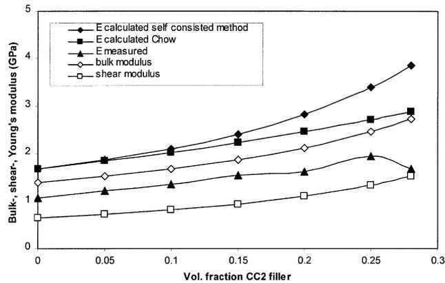
Fig. 21. Experimental measurements of the dependence of the Young's moduli compared with predictions made from the self consistent method and the Eshelby inclusion method.
