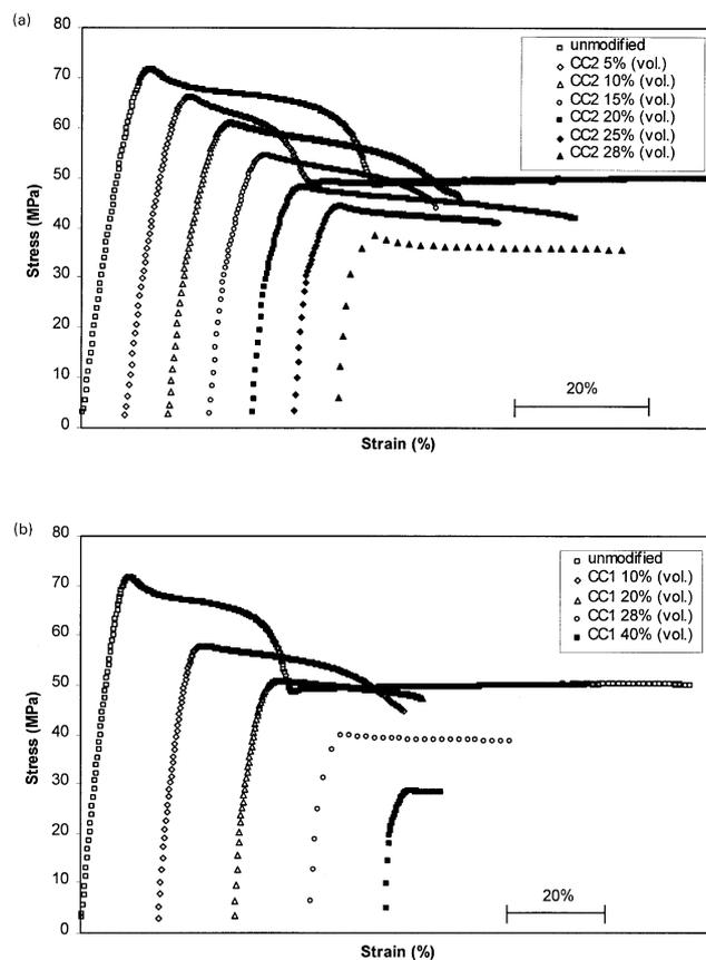
Fig. 1. Stress-strain curves of the series of Nylon-6 with (a) CC2 and (b) CC1 fillers. Tests were performed at  $20^{\circ}\text{C}$ . Each curve was shifted along the strain axis for clarity.
