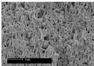
Fig. 14. SEM micrograph taken 0.9 mm below the fracture plane of the blend with 0.25 volume fraction of CC2 filler.
