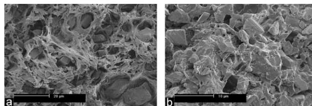
Fig. 12. SEM micrographs of the fracture surface of the tensile bar of the Nylon-6/CC1 blend with 0.1 of filler: (a) a ‘ductile’ region and (b) a brittle region.
