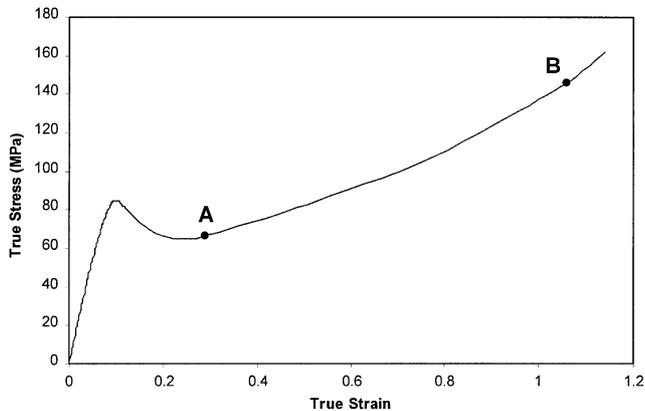
Fig. 24. A tensile true-stress/true-strain curve for unmodified Nylon-6.
