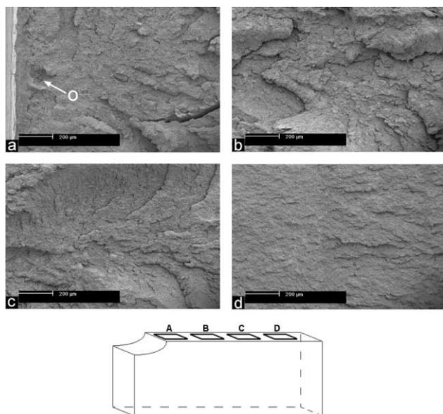
Fig. 17. SEM fractographs of the broken Izod sample of the Nylon-6/CC2 blend with 0.15 of CC2 filler. The fractographs were taken at increasing distances from the root of the notch, taken at distances of respectively: 0.3, 2.5, 5.0 and 7.5 mm from the root of the notch, as depicted in the attached sketch. The crack propagated from left to right.
