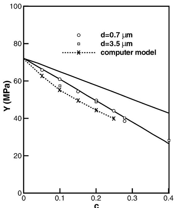
Fig. 26. Dependence of the yield stress on particle concentration: experimental values, upper bound calculations and computer model results.
