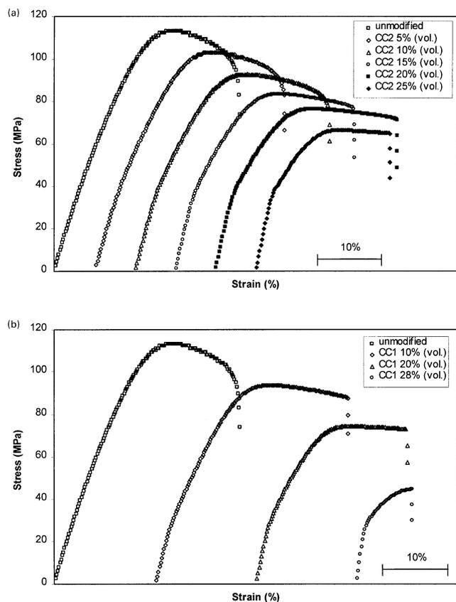
Fig. 4. Stress–strain curves of the series of Nylon-6 with (a) CC2 and (b) CC1 fillers. Tests performed at  $-30^{\circ}\text{C}$ . For clarity each curve was shifted along the strain axis.
