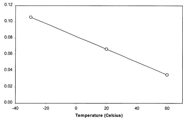
Fig. 25. The temperature dependence of the yield stress normalized with the appropriate Young's modulus.
