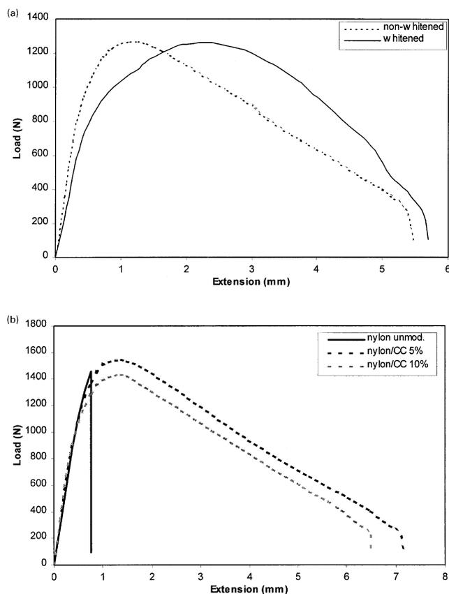
Fig. 7. (a) Load-extension curves of the whitened and non-whitened SECP specimen from the Nylon-6/CC blend with 0.15 of CC2. The tests were performed at 20°C at a crosshead speed of 5 mm/min. (b) Load-extension curves of the non-whitened SECP specimens from the unmodified Nylon-6 and the Nylon-6/CC2 blend with 0.05 and 0.10 filler respectively. The tests were performed at 20°C at a crosshead speed of 5 mm/min.
