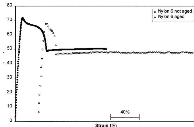
Fig. 2. A comparison between the stress–strain behavior of the unmodified Nylon-6 from the batch form 1997 and 2000. The curves are shifted for clarity.
