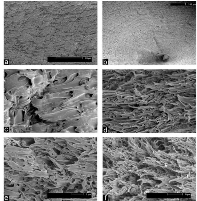
Fig. 10. SEM fractographs of the fracture surfaces of tensile bars of Nylon-6/CC2 blends: (a) no filler, (b) 0.05, (c) 0.05 at higher magnification, (d) 0.1, (e) 0.15, (f) 0.2 filler. In the higher magnification fractographs the direction of crack propagation is from right to left.
