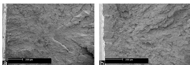
Fig. 18. SEM fractograph showing fracture origins of the Izod impact samples of the Nylon-6/CC2 blend with (a) 0.1 of CC2 filler and (b) 0.25 of CC2 filler. The root of the notch is visible in the left side of the pictures.
