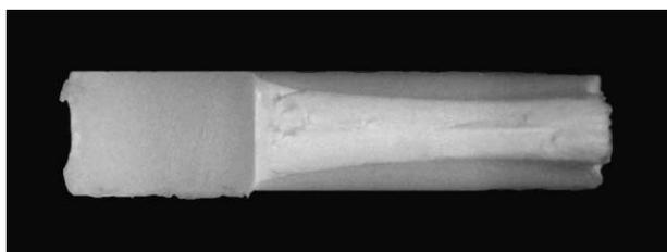
Fig. 8. Reduction of cross-sectional area in the SECP specimen of the Nylon-6/CC2 blend with 0.1 filler.
