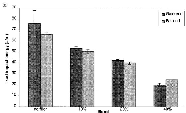
Fig. 5. Notched Izod impact energies measured at 20°C for (a) unmodified Nylon-6 and Nylon-6/CC2 blends; (b) pure Nylon-6 (no filler) and Nylon-6/CC1 blends. Izod impact energies for gate end and for far end specimens are shown separately.
