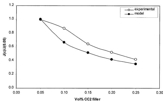
Fig. 29. Calculated normalized fracture toughness compared with experiments.
