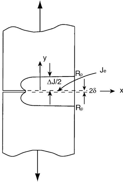
Fig. 28. Sketch of the whitened zones of the SECP specimens.
