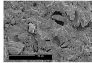
Fig. 15. SEM micrograph taken 3.0 mm below the fracture plane of the blend with 0.20 of CC1 filler.
