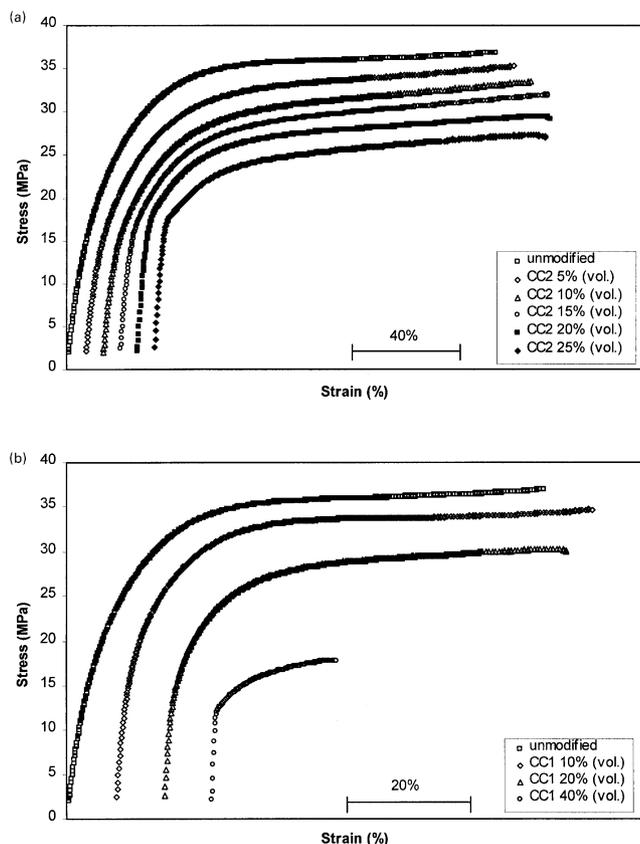
Fig. 3. Stress–strain curves of the series of Nylon-6 with (a) CC2 and (b) CC1 fillers. Tests were performed at 60°C. For clarity each curve was shifted along the strain axis. The unmodified Nylon-6 and the blend with volume fraction of 0.10 of CC1 did not break. The blends with volume fractions of 0.05, 0.10 and 0.15 of CC2 also did not break.
