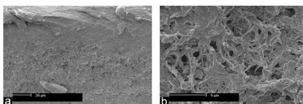
Fig. 20. SEM cryo-fractograph in the Izod-1 plane of the Izod impact specimen of the Nylon-6/CC2 blend with 0.10 of CC2 filler, just below the surface: (a) at low magnification; and (b) at high magnification.
