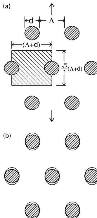
Fig. 27. A 2-D model of the CC particle distributions in the matrix: (a) before deformation, (b) after debonding during loading to yield stress showing particle separation at the poles.
