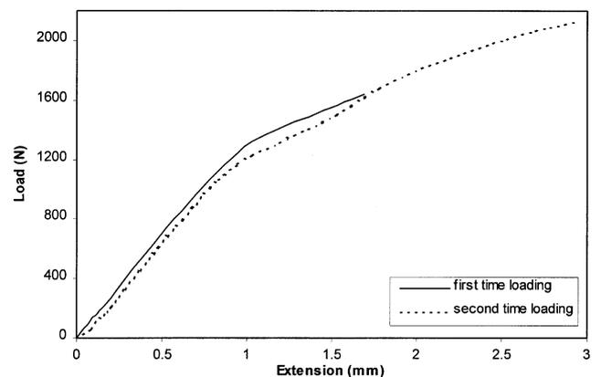
Fig. 23. Reversible particle debonding behavior. Solid curve gives initial response. Dotted curve gives response on re-loading.
