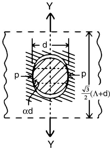
Fig. 30. Sketch of incompletely separated particle, producing triaxial tensile stress.
