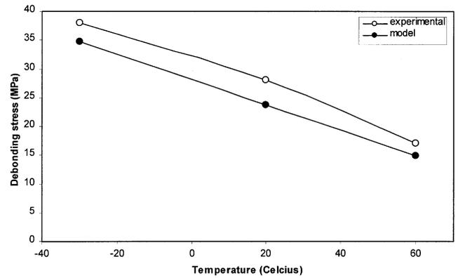
Fig. 22. Temperature dependence of the debonding stress: experiments and model prediction.
