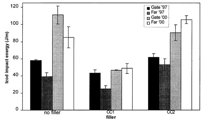
Fig. 6. Notched Izod impact energies measured at room temperature for the blends prepared in 1997. These blends all contain 0.28 volume fraction of CC filler. One pair of gate end and far end Izod impact energies was measured in 1997. The other pair of Izod impact energies was measured in 2000.
