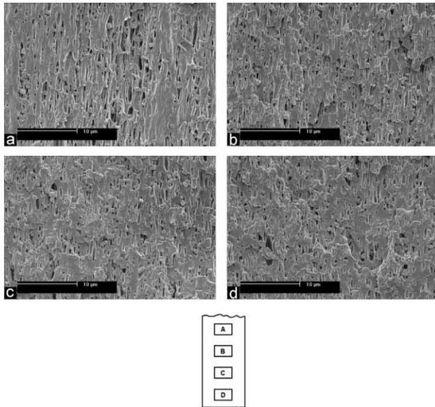
Fig. 13. SEM micrographs of the bulk of the tensile bar of the Nylon-6/CC2 blend with 0.1 of CC2 filler. The distances away from the crack plane of the region of the micrographs are depicted in the attached sketch and are at distances of: 0.1, 0.8, 1.5 and 2.2 mm, respectively below the fracture plane.
