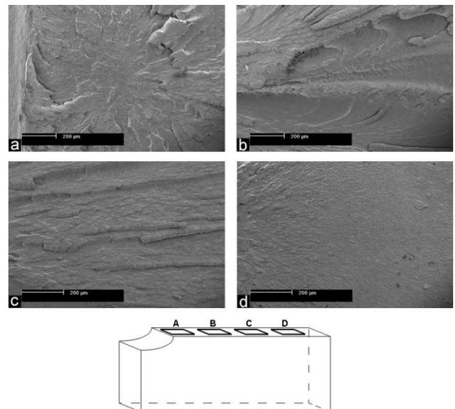
Fig. 16. SEM fractographs of the broken Izod sample of unmodified Nylon-6. The fractographs were taken at increasing distances away from the root of the notch at: 0.3, 2.5, 5.0 and 7.5 mm from the root of the notch as depicted in the attached sketch. The crack propagated from left to right.
