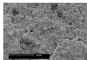
Fig. 19. SEM fractograph of the cavitation on the Izod impact specimen fracture surface of the Nylon-6/CC2 blend with 0.15 of CC2 filler.
