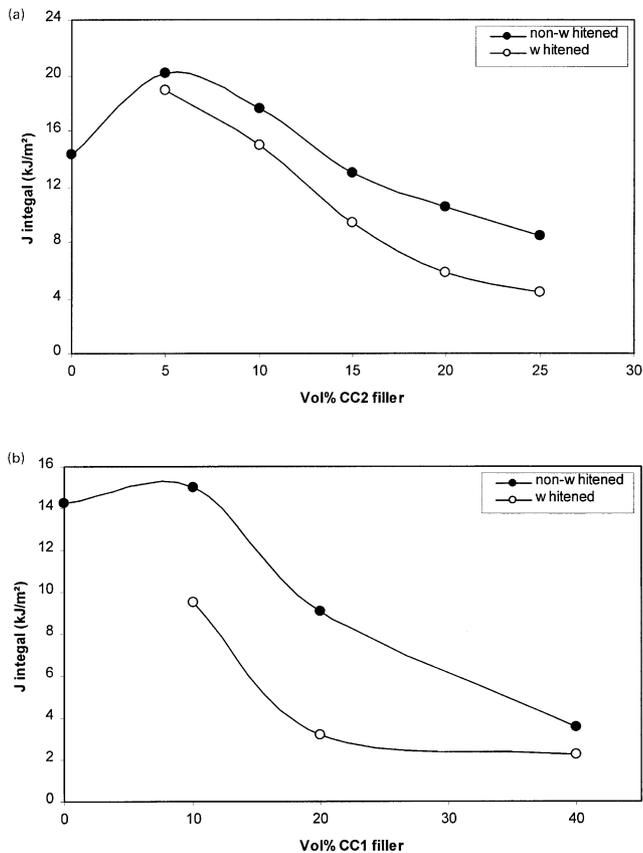
Fig. 9.  $J$  integral value of different Nylon-6/CC blends plotted against the volume fraction of CC filler: (a) for CC2 filler, and (b) for CC1 filler. The tests were performed at 20°C and a cross head speed of 5 mm/min.
